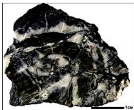
Figure 8 - Zone of crumpling with maximum conversion of carbonaceous matter in sliding mirrors. Grinding-in.
