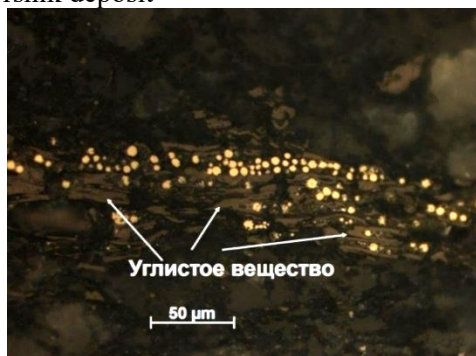
Figure 5 - Globular pyrite (bright balls) in carbonaceous matter. Bakyrshik
