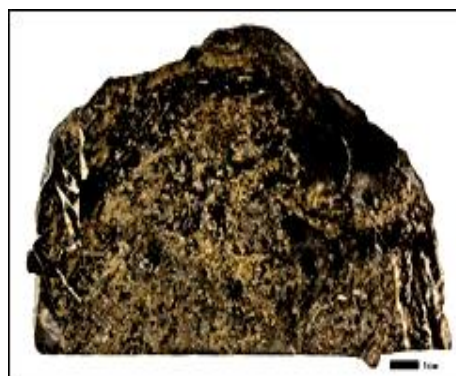
Figure 9 - Distribution of pyrite and arsenopyrite mineralisation and quartz cuttings in carbonaceous-enriched boudin. Sample.
